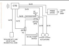
**Operation:** Presenting a valid credential to Schlage MT XX-485 will cause QEL panic device to retract for authorized entrance and enable exterior actuator. Free non-alarmed egress at all times. Interior actuator always active to retract QEL panic and open door.
