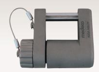
steel to withstand severe physical attack. Each padlock includes a weather seal cap attached by a cable. The Medeco® G8R will accept either an eCylinder or mechanical t-handle cylinder. The mechanical cylinders provide the benefit of patented key control and pick resistance. The eCylinder adds sophisticated audit and control features transforming the G8R into a portable access control system for extreme environments.
